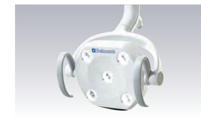
300 LED light The 300 LED light provides sensor activation, stepless intensity between 3100 lx and 28000 lx, three axis rotation and clear light pattern. Composite safe mode at 4300 lx.
