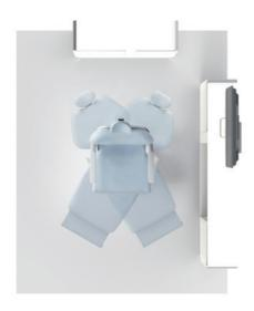
The chair rotates on its base left-to-right so patients can be repositioned for taking X-rays for treatment procedures. The chair's small footprint in the upright position requires less space within the surgery.
