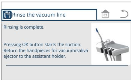
3. After rinsing of the vacuum line is completed, press the **OK** switch.
