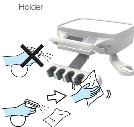
Wipe the surface with a soft cloth or paper towel moistened with FD366 manufactured by Dürr, and then wipe it with a dry cloth.
