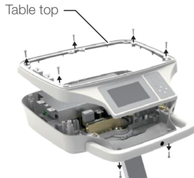
2. Remove the seven screws and detach the table top.
