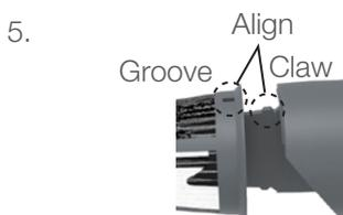
5. Align the claw on the solid collector cap with the groove on the filter to attach them.
